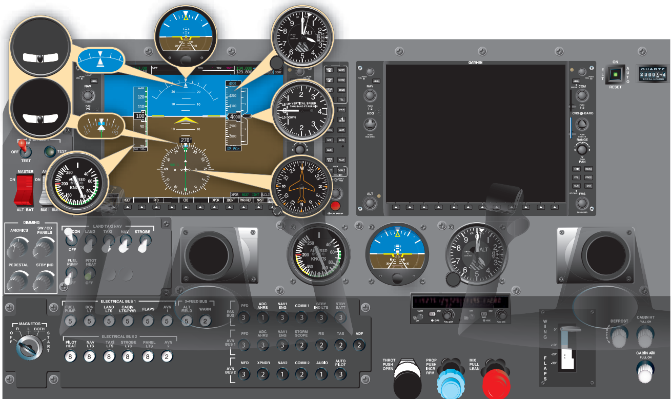
Figure 6-21. Primary flight display (PFD) and analog counterparts.
