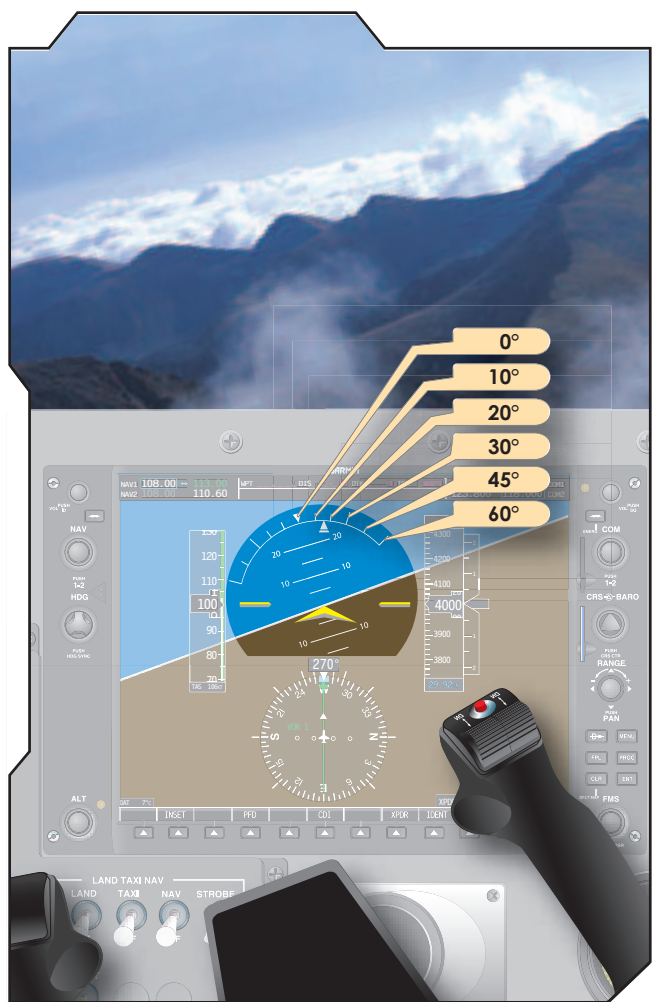
Figure 6-29. Bank indicator index lines.
