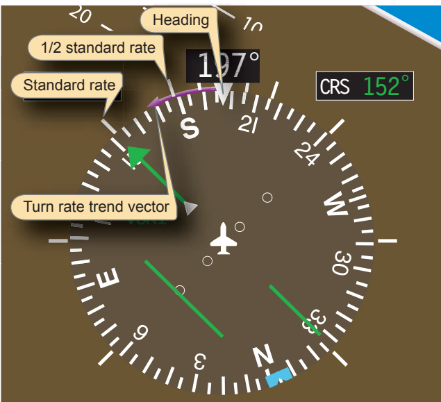
Figure 6-39. HSI indicator (enlargement).
