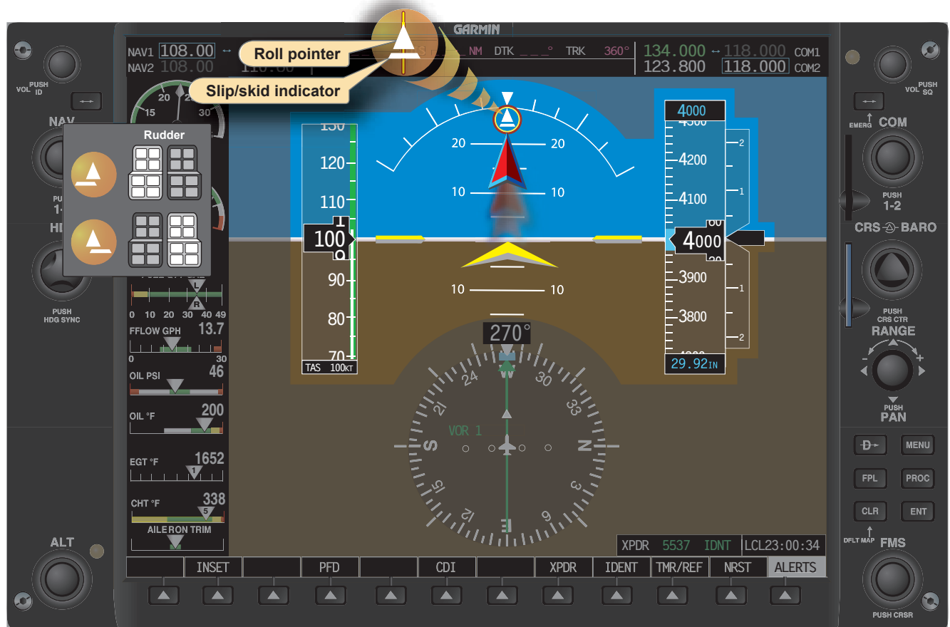
Figure 6-34. Roll pointer and slip/skid indicator.
