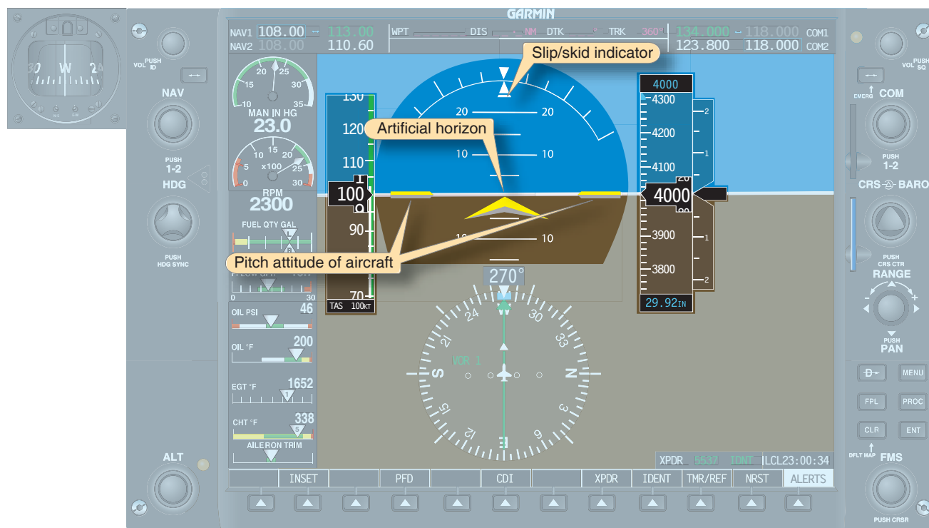
Figure 6-30. Pitch of the aircraft.
