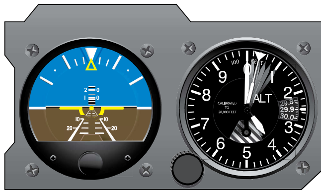
Figure 6-7. Pitch correction using the altimeter.
