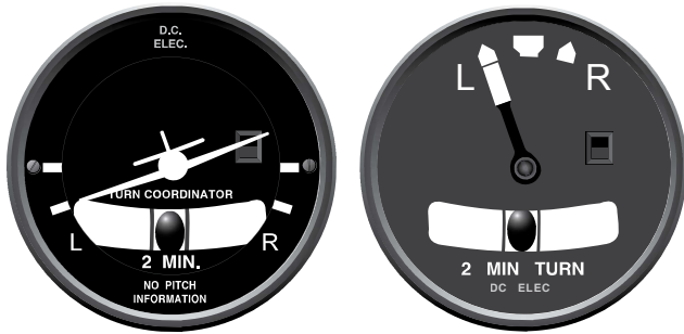
Figure 6-12. Turn coordinator and turn-and-slip indicator.
