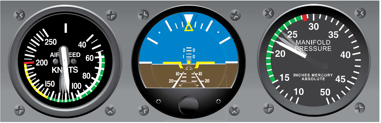
Figure 6-14. Pitch control and power adjustment required to bring aircraft to level flight.
