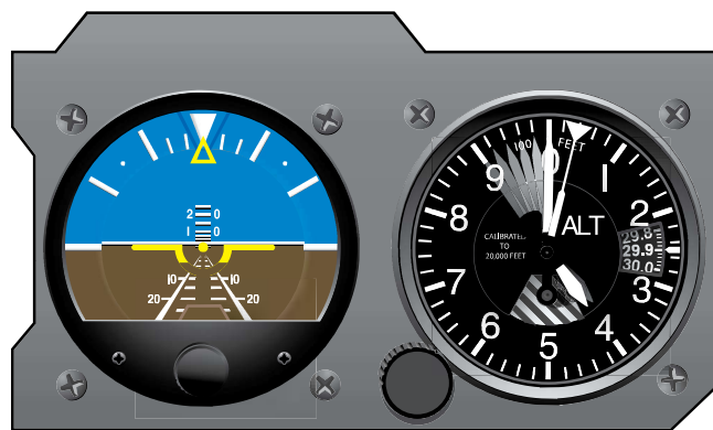
Figure 6-6. Pitch correction using the attitude indicator.
