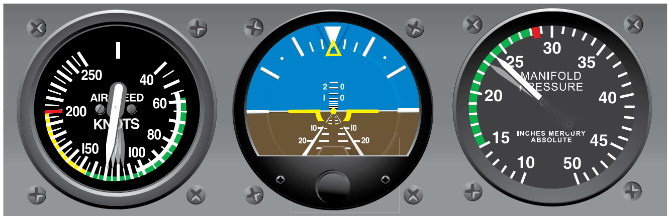
Figure 6-13. An increase in power—increasing airspeed accordingly in level flight.
