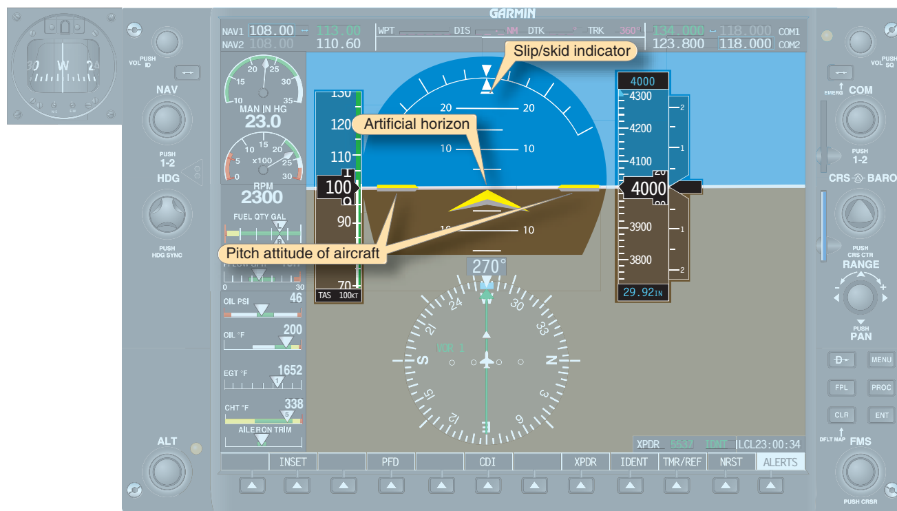
Figure 6-30. Pitch of the aircraft.
