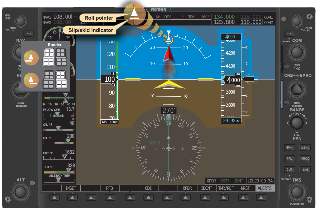
Figure 6-34. Roll pointer and slip/skid indicator.
