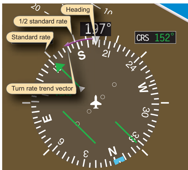
Figure 6-39. HSI indicator (enlargement).
