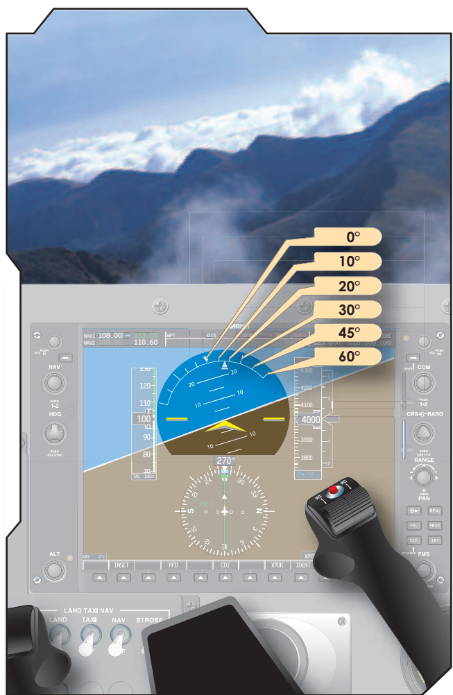
Figure 6-29. Bank indicator index lines.
