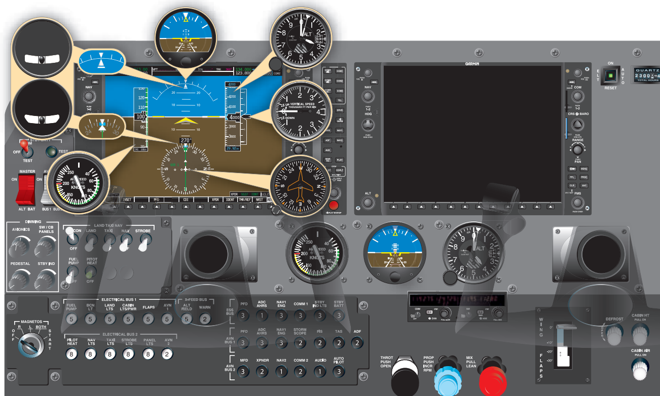
Figure 6-21. Primary flight display (PFD) and analog counterparts.
