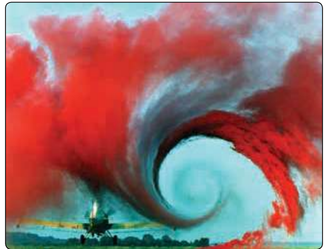
Figure 5-9. Wingtip vortex from a crop duster.
